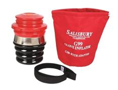
**Description:** The G99 is a simple, easy to use, portable glove inflator. The G99 provides a quality means of inspecting gloves in the field. The glove is secured to the inflator using a nylon strap and fastened with a hook and pile closure. Inflation is accomplished by pumping the bellows of the inflator against any surface.
